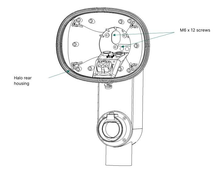
Use the 3 pcs M6 x 12 screws in the installation kit to attach the Halo rear housing to the Halo Pole Mount. Remember to put the gasket from the halo package in between the halo rear housing and the Halo Pole Mount.
