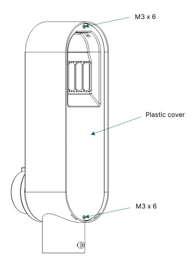
Unscrew the two M3 x 6 screws, remove the plastic cover and put aside.
