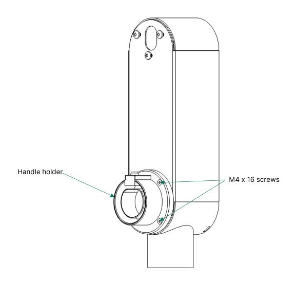
Mount the handle holder on Halo Pole Mount using the 4 pcs M4 x 16 screws in the installation kit.
