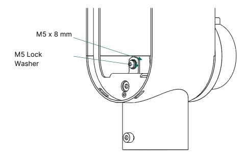
Use M5 Screw / Washer to secure the Ground wire for the Pole Mount Chassi
