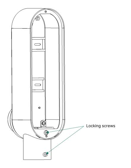
Put the Halo Pole Mount in position on the pole and tighten the two locking screws.
