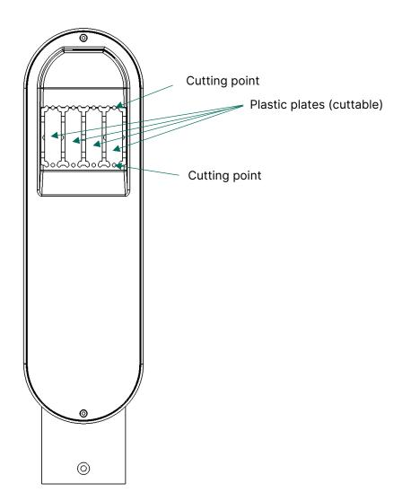
The plastic cover has four plastic plates that can be cut off if an earth leakage circuit breaker, ELCB, will be used. Measure the ELCB and cut away the plastic plates corresponding to the width. Cut the plates after the plastic cover has been removed and put aside, described in the picture below.
