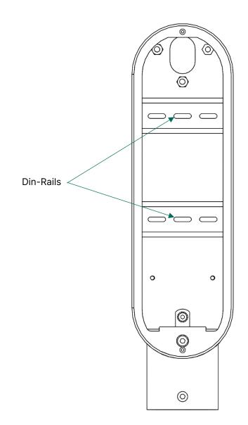
There will be two Din-rails preinstalled for potential add ins, such as a terminal block, EFCB etc.
