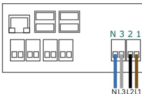
Figure 6 Power supply connected to Measurement Device
