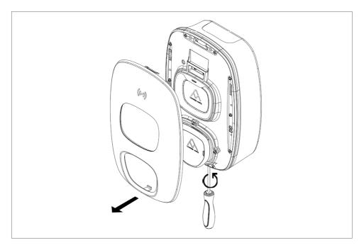
2. Remove the front cover by a pull from the bottom.
